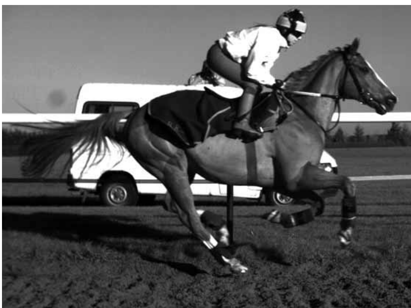
A Board funded research project by Professor Alan Wilson, Royal Veterinary College, into the relationship between surface properties and factors predisposing to injury in the racehorse. The horse is at full gallop with a wirelessly synchronized system for measuring the horse/surface interaction. A GPS unit on the rider's helmet tracks speed and position, and accelerometers on the hooves measure impact decelerations. Photograph: courtesy of Professor Alan Wilson, Royal Veterinary College.
